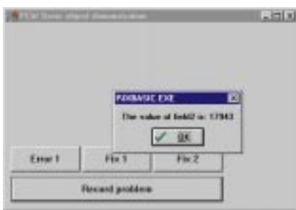
Fig 4 When you use a record type variable, you must initialise its values. Otherwise you get random results like this one
